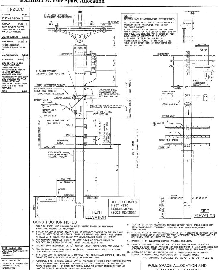
FIELD MANUAL #9 OVERHEAD CONSTRUCTION SECTION 5: POLE INSTALLATION
