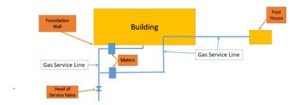
Note: The purpose of this diagram is to depict the jurisdiction of Gas Service Line vs. Customer Piping. It does not identify areas along the Gas Service Line for which the customer is responsible, per Con Edison's tariff agreements.
