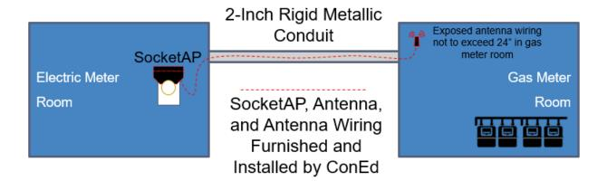
F. Meters must communicate with each other and, ultimately, to access points (AP) or socket access points (Socket APs) using a mesh radio frequency network. All Socket Access Points (Socket AP) act as the communications link to transfer meter data back to Con Edison.
