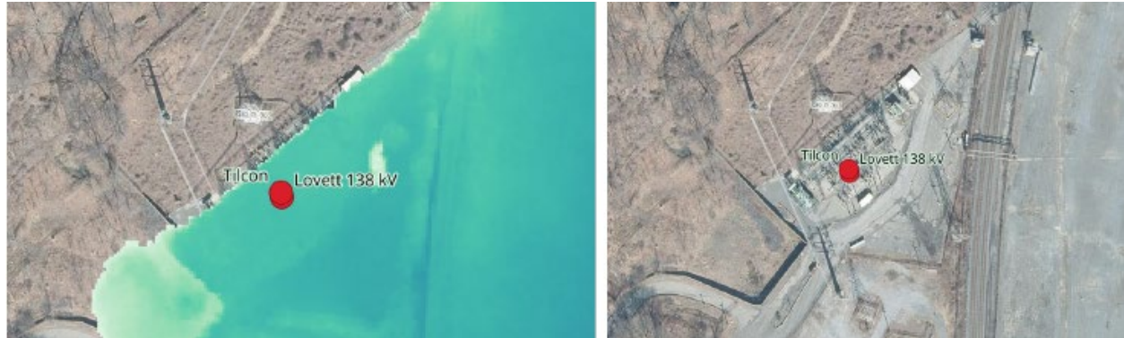
Figure 2. Lovett 138kV substation yard shown with and without inundation from the FEMA 100-year flood plain extent due to the Hudson River.
