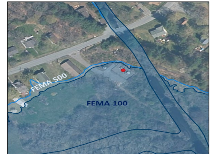
Figure. Summitville substation (red point) with the FEMA 100- and 500-year floodplains overlaid
