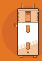
Heat pump water heaters extract heat from the air surrounding the unit to heat water. They can replace electric or fossil fuel-powered water heaters that require much more energy to run efficiently—leading to big savings.
